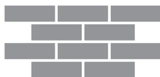
If you can't see the pattern of the brick work then measuring the thickness of the wall at any entrance or window will help to determine the construction type. A solid brick wall is usually about 22 cm thick, a cavity wall between 27 cm and 30 cm thick, and a solid stone wall could be as much as 50 cm. The age of your home can also be a good indicator. As a general rule, if it was built before the late 1920s it is unlikely to have a cavity.
